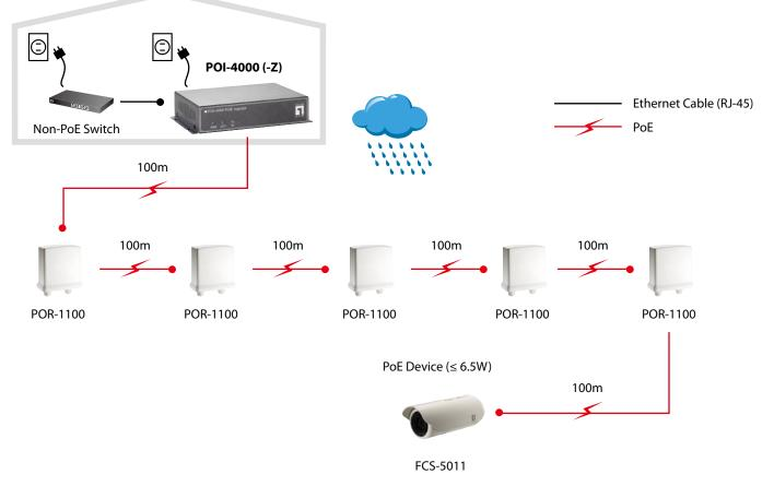
Note: These distances are typical results when used with 18~19 $\Omega$  24 AWG Cat.5 Cable
