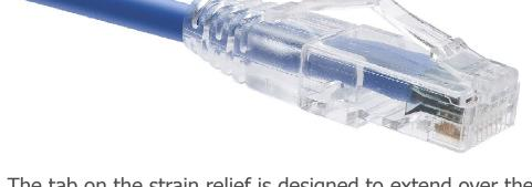
The tab on the strain relief is designed to extend over the plug's locking tab, making it snag proof when administering patch cords. The primary strain relief of the plug locks the snag proof strain relief in place so they will not pull off, creating one, integral assembly. Once crimped, this design allows the plug's primary strain relief to relax slightly, preventing the cable pairs from being over compressed. This decrease in stress contributes to achieving peak performance.
